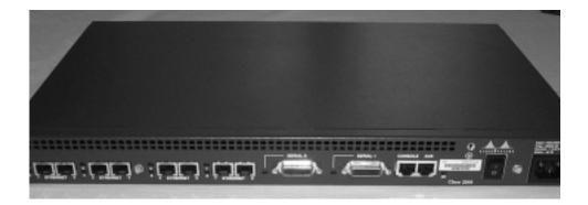
Cisco routers, such as those in the 2500 Series family, are off-the-shelf routers that come with a predetermined number of LAN, WAN, and serial ports. Higher-end routers like the Cisco 4500 are modular and actually contain empty slots that can be filled with several different interface cards.
