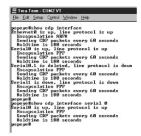
You can also view the CDP information for a particular interface. For example, in the screen shot above, the command that follows the initial **show cdp interface** command is **show cdp interface s0**. This provides the CDP information for just interface serial 0.
