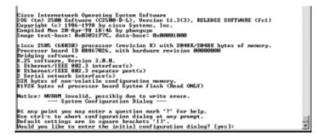
Working through the Setup dialog is very straightforward. You will need to know certain parameters related to the configuration of the router, such as which network protocols you will route (IP, IPX, AppleTalk, etc.) and the parameters related to the various interfaces.
